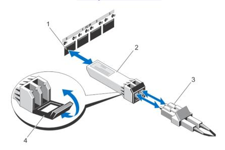
Figure 7. Installing and Removing an SFP Module
